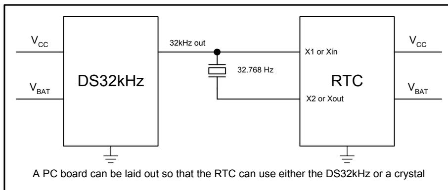
**Figure 6. DS32kHz and RTC Connections**
