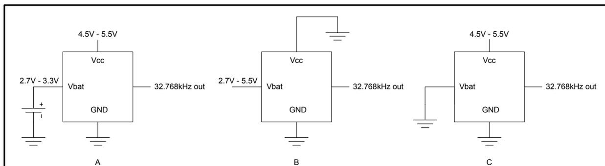
[Figure 5](#) illustrates how a standard 32.768kHz crystal and the DS32kHz should be connected to address the interchangeable option. Using this connection scheme and the recommended layout provides a solution, which requires no hardware modifications. Only one device should be used at a time, and both layouts should be located very close together if the recommended layout is not used.
